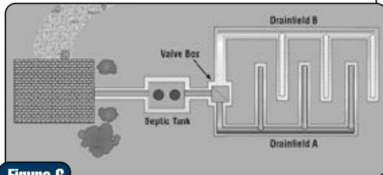
**Figure 6** Interlacing drainfields.
