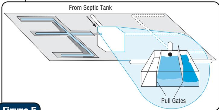
**Figure 5** Alternating drainfields.
